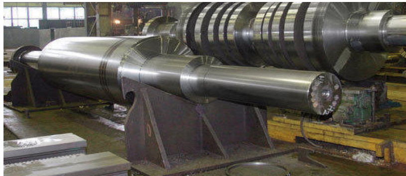
Figure 3.10 Turbine Generator Shaft Rs 1.25 Lakh
